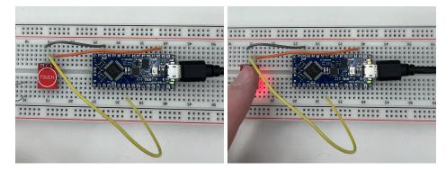
To test the functionality of the touch sensor, we developed a simplistic code system that, upon pressing the button, turned on the onboard LED (seen top right with a yellow glow) for one minute before turning it off. This doubled as a test for the Arduino's timer system we would need later.
