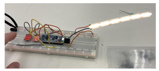
The next test was finding the currents that would be drawn by the Arduino Nano and making sure that the outputs were working as intended. These need to be found so the overall current draw can be calculated to find the correct battery. Along with that, the output voltages of the I/O were also found.
